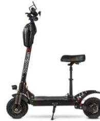
StreetScan has developed a scooter-based approach which captures all the necessary distresses. StreetScan utilizes high resolution 2D imaging technology to collect sidewalk video, and identify distresses such as cracks, surface distortions, general uplifts, and tree uplifts. A mobile phone and high-grade GPS device are used for controlling data collection.
